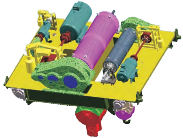
Double girder overhead crane traversing trolley
