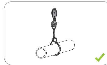
Figure 9: Prevent fouling of safety latch on load. Sling in base of hook.
